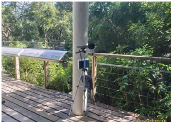
Air quality and noise monitoring at Noise Sensitive Receiver (NSR)
