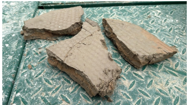
Sludge “cake” after dewatering
